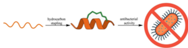
Fig.1. Schematic representation of the structure–activity relationship for membrane-active peptides. Hydrocarbon stapling stabilizes the \alpha -helical conformation of unstructured, linear peptides thereby conferring antibacterial activity.
